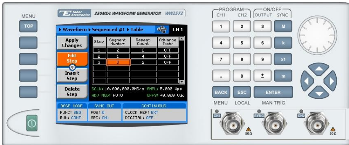
Figure 1-17, Typical Front Panel Programming of a Sequence Table
