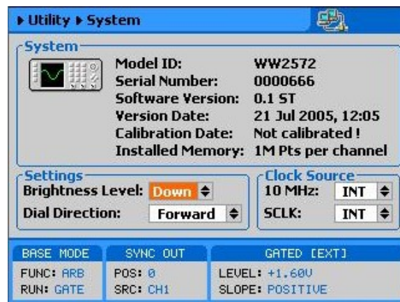
Figure 3-13, Modifying the SCLK and 10MHz Clock Source
